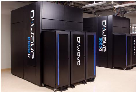
Figure 26.8: D-wave's room-sized 2000-qubit quantum annealing device.
